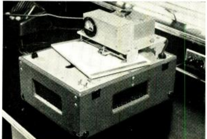
Fig. 5. The polinear recorder used for plotting polar diagrams. Deflection of pen is proportional to the signal being received.
