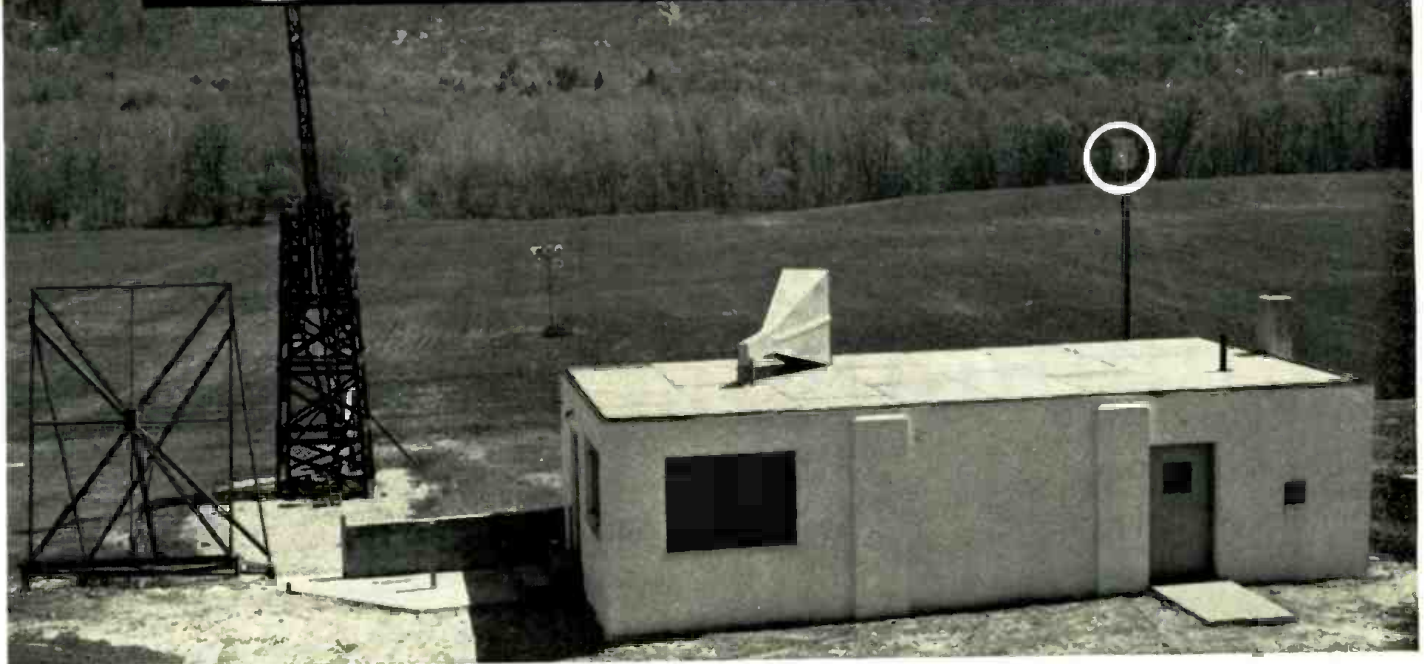
Fig. 1. Channel Master's Antenna Laboratory. Left is v.h.f. range showing broadband corner reflector transmitting antenna with receiving tower (large circle) in background. The u.h.f. horn transmitting antenna is on roof with receiving mast (small circle) at rear of building.
