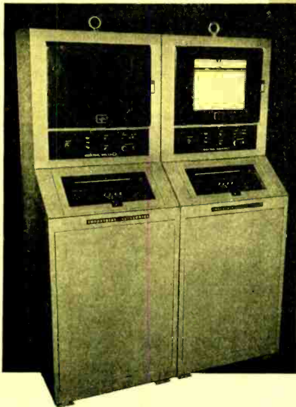
Fig. 1. Consoles which house the electronic circuitry for dual beta gauge installation.
