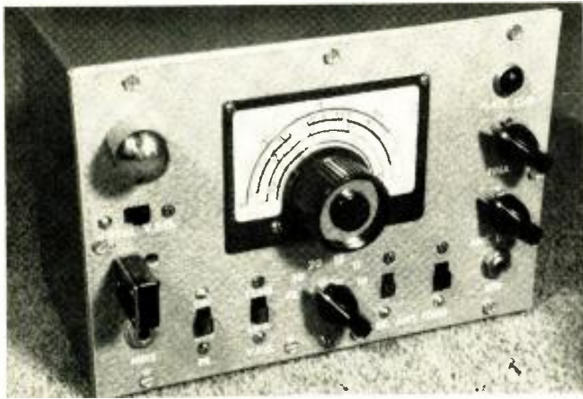
Fig. 2. All controls but the phone-c.w. switch are located on the front panel. Note that several extra self-tapping screws are used to fasten the panel, improving rigidity for the v.f.o.
